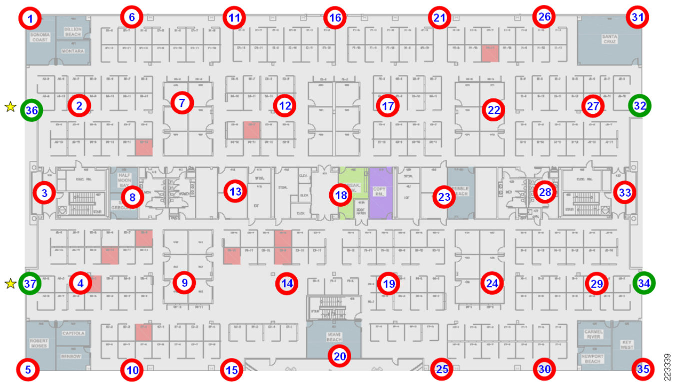
Figure 5-21 Layout for 5GHz Voice and High Speed Data, 2.4GHz Legacy, with Location
