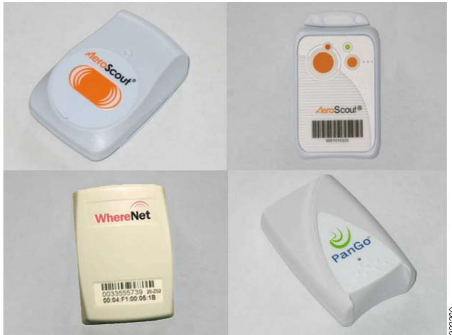
Figure 6-9 802.11 Wi-Fi Active RFID Tags
