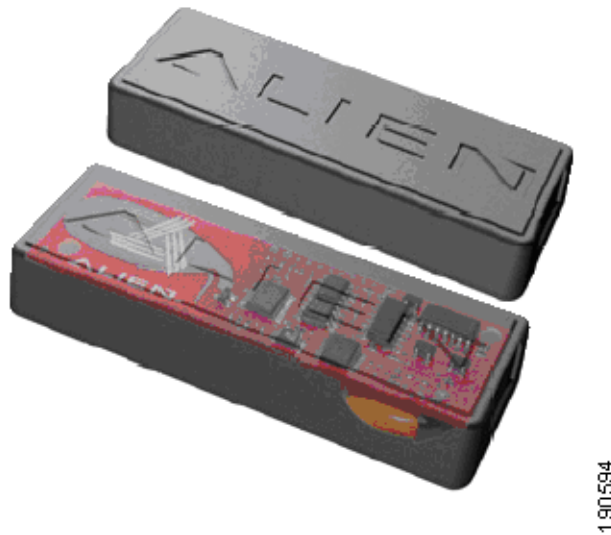
Figure 6-7 Semi-Passive RFID Tags
