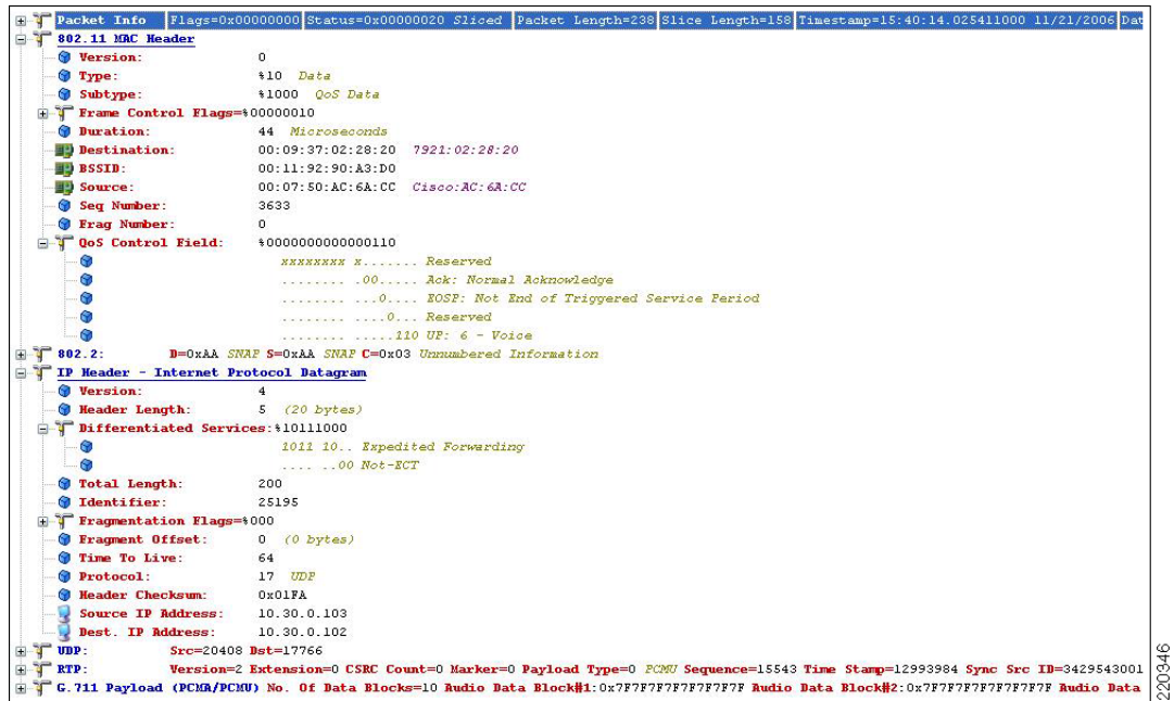
Figure 9-10 Sample VoWLAN Capture
