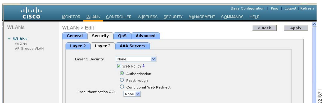
Figure 10-21 Guest WLAN Layer 3 Security Configuration
