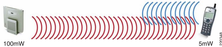
Figure 9-14 Client and AP Power Matching
